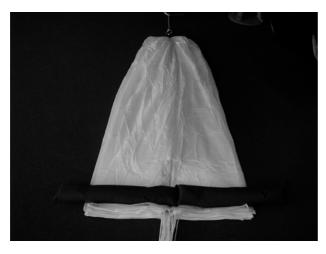
Lay down the canopy so that there are the same numbers of panels on each side (keep the canopy under tension). Use sand sacks to weight down the base of the canopy.
